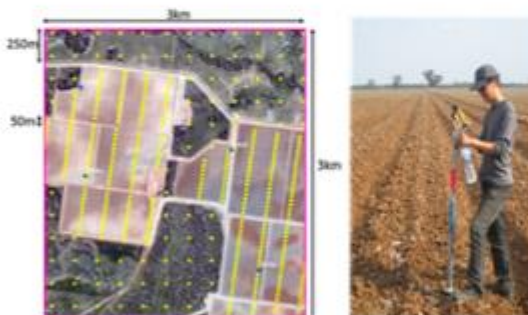
Fig. 2: Field technician with soil moisture probe and schematic of a possible sampling points distribution across a farm.
