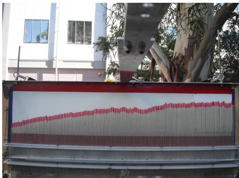
Figure 6-3. Pin profiler for surface roughness measurements.
