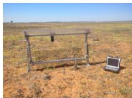
Fig. 4: Surface roughness sampling using a laser-pin board profiler.
