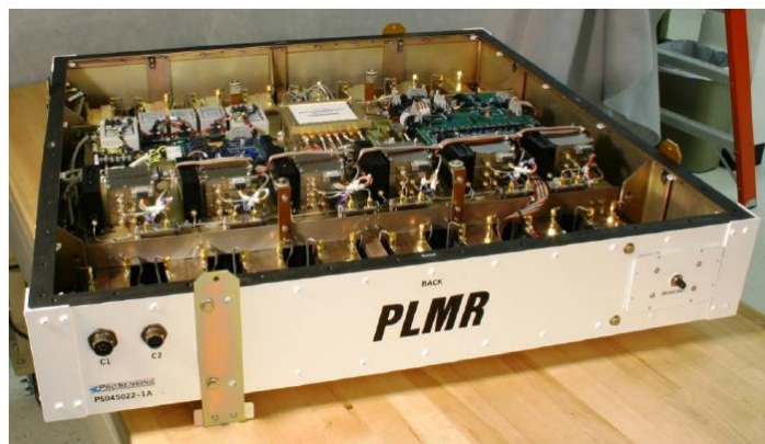
Figure 2-3. View of PLMR with the cover off.
