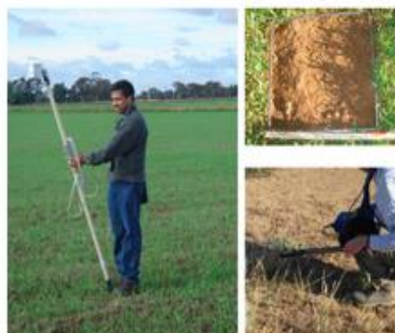
Fig. 3: Typical vegetation sampling within a 50cm × 50cm area and example of non-destructive spectral measurements.
