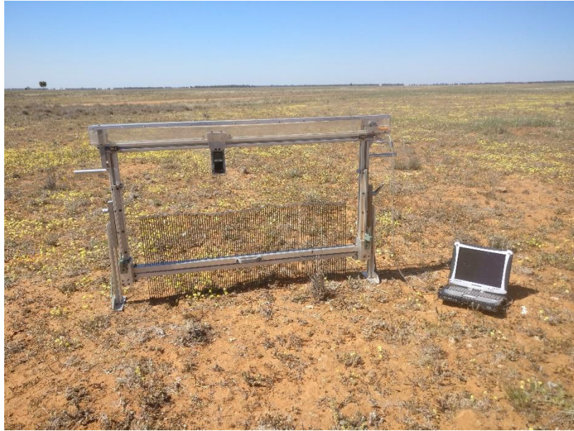
Figure 6-5. Laser-pin profiler for surface roughness measurements.
