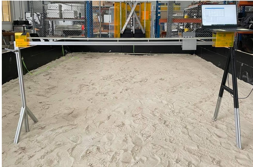
Figure 6-4. Laser profiler for surface roughness measurements.
